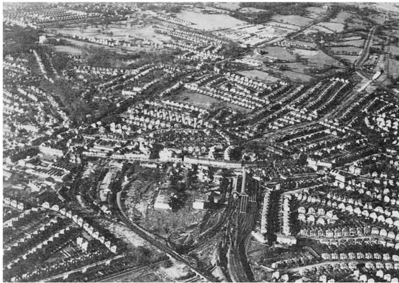
(Plate 2.6) Edware, north-west London: (a) 1926; (b) 1948, showing the impact of the extension of the underground railway (station in centre of pictures) on suburban development. Typical are the uniform rows of semi-detached housing, built at about 12 dwellings to the acre (30/hectare), with generous gardens. Better transportation allowed the city to spread.
